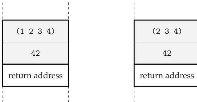
One way to observe the effects of TCO is to look at the output of the disassembler (see Recipe 17-12). On x86, a function call would usually appear as `call` but would be replaced by a `jmp` instruction in case of tail call elimination.
