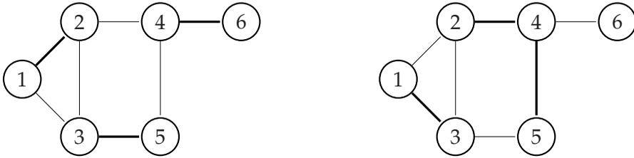
In the picture on the left, the set of thick edges is  $\{\{1,2\}, \{3,5\}, \{4,6\}\}$  and it is a matching. In our program we'll represent it<sup>40</sup> as the list  $((1\ 2)\ (3\ 5)\ (4\ 6))$ . The set of thick edges on the right is  $\{\{1,3\}, \{2,4\}, \{4,5\}\}$ , which is *not* a matching as two of the edges coincide with the vertex 4.
