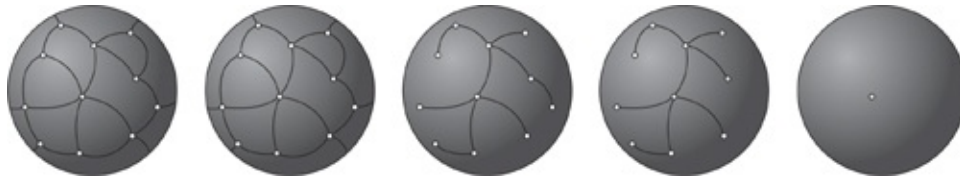
Fig 21 Key stages in simplifying a solid. Left to right: (1) Start. (2) Merging adjacent faces. (3) Tree that remains when all faces have been merged. (4) Removing an edge and a vertex from the tree. (5) End.
