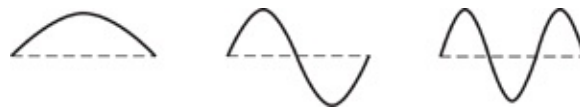
Fig 36 Snapshots of modes 1, 2, 3 of a vibrating string. In each case, the string vibrates up and down, and its amplitude varies sinusoidally with time. The more waves there are, the faster the vibration.
