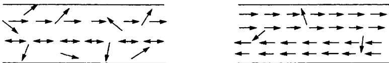
FIGURE 20.5.31 Illustration of the growth of the stimulated emission probability with the intensity of the mode.
