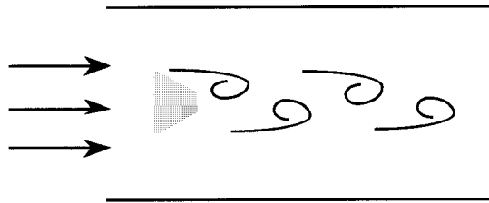
FIGURE 3.13.10 Vortices shedding off a body placed in a moving stream.
