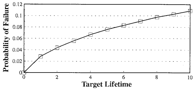
FIGURE 1.6.32 Example FAROW results for probability of premature failure as a function of target lifetime. (Courtesy Sandia National Laboratories, Albuquerque, NM.)
