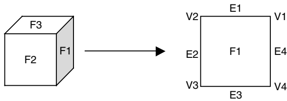
FIGURE 11.3.6 Basic concept of the B-Rep model.
