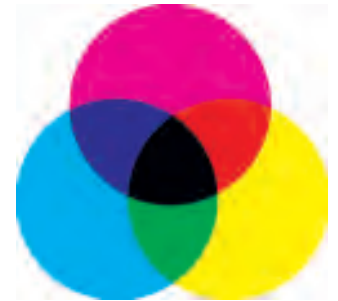
Figure 5. The primary colors of a subtractive color system and their combinations.
