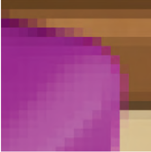
Figure 24. Antialiasing example. Pixels at the edges of objects are blended into the background colors.
