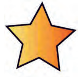
Figure 14. The orange to yellow star, severely quantized to illustrate banding or contour lines. Normally, quantization effects are more subtle.
